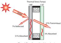
Tinted Glass (heat-absorbing glass) ¼" gray float glass outboard / ¼" clear inboard Tvis = 42% SHGC =0.48
