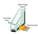
while offering varying levels of structural integrity that may or may not be suitable for commercial applications. Warm-edge spacers can significantly reduce heat conduction when compared to conventional metal spacers.
