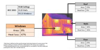
Upgrades in glazing technology in the last 20 years have significantly improved heat-loss performance for residential and commercial structures.
